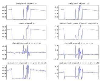
The above shown graphs are the main differences between the classical and generalized unsharp masking algorithm. Here we show the clear difference between the addition and generalized addition. And at last we show that the enhancement is more in generalized unsharp masking algorithm rather than in classical unsharp masking algorithm.
